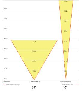
In lighting, choosing the lens angle is as important as selecting the color or wattage. Small angles retain brightness at long distances, while wide angles cover larger areas but lose brightness over distance.
